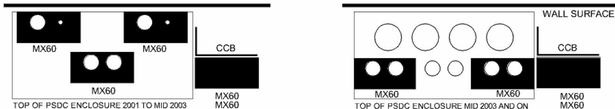
Figure 2. Three MX60 mounting options on the top of an OutBack PSDC Disconnect Enclosure
