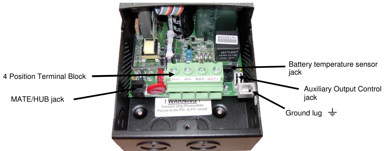
Figure 3. MX60 wiring area and wiring terminals
