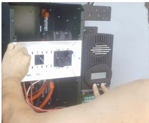
Setting system Voltage with the “Mind Meld”
